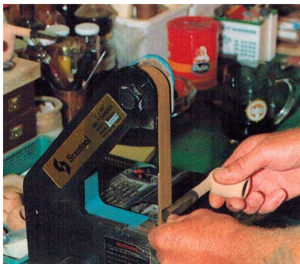
The small belt sander is used for the stem work
