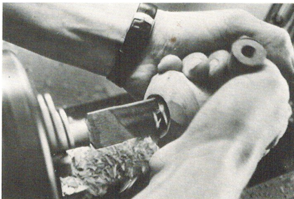
The chamber is drilled on the lathe "by hand". Notice the drill, - it is homemade from an old file
