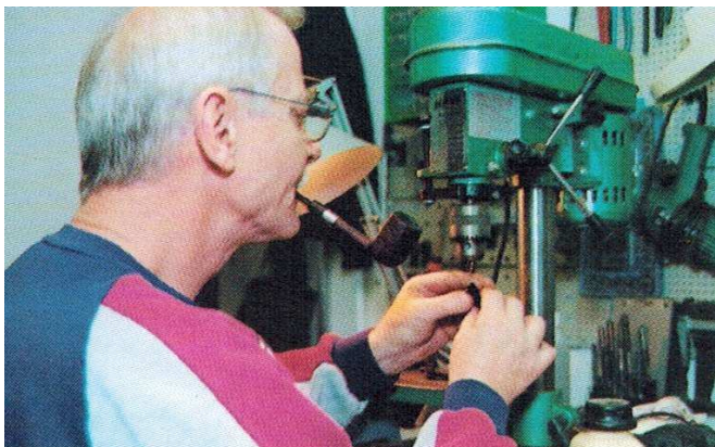
Finn milling the smoke channel
