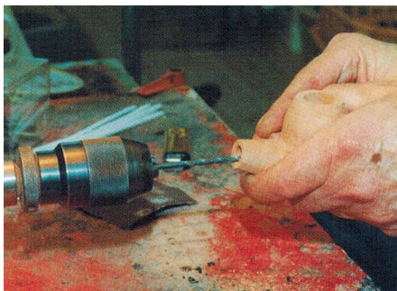
A half-bent modelis being drilled. This is why the drill bit is placed low in the mortise.
