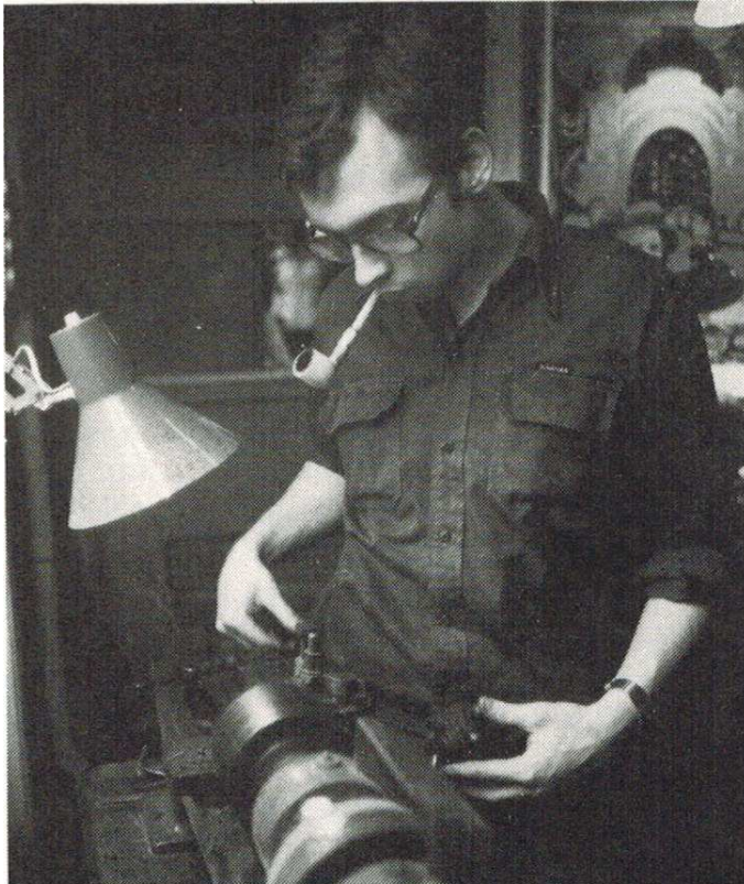
Deep concentration while the stem is turned to match the bowl
