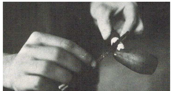
Stain is applied to the bowl using a pipe cleaner
