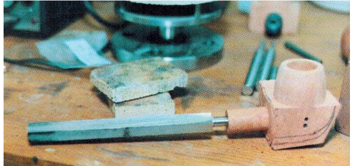
The master for milling facet pipes is made by Finn
