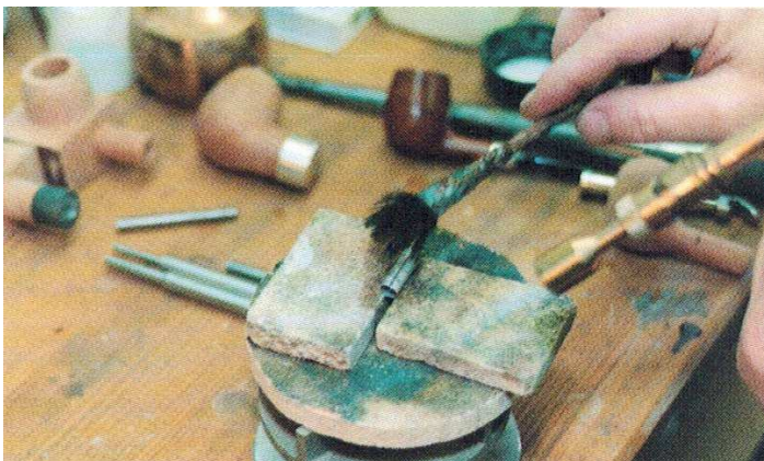
Flux is applied to the silver
