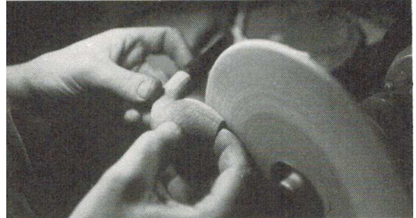
The model is shaped on the sanding wheel "bims".
